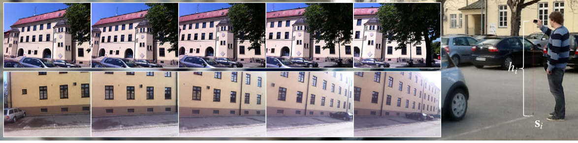
Figure 4.8: Sequence recording at a known camera position using a lead weighted string and measured survey points on the ground.
