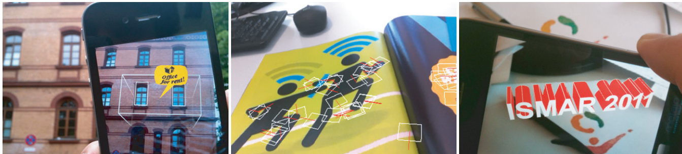
Figure 1: Gravity-awareness in handheld AR: detecting vertical surfaces, such as building façades, improves when using gravity-aligned feature descriptors (GAFD) [12] (left). For horizontal surfaces, such as a magazine on a table (center), we introduce gravity-rectified feature descriptors (GREFD) that describe a feature based on a gravity-rectified camera image. We also show, how inertial sensors enable full 6 DoF pose estimation from horizontal surfaces with an occlusion-invariant edge-based detection method that only supports similarity transforms (right).
