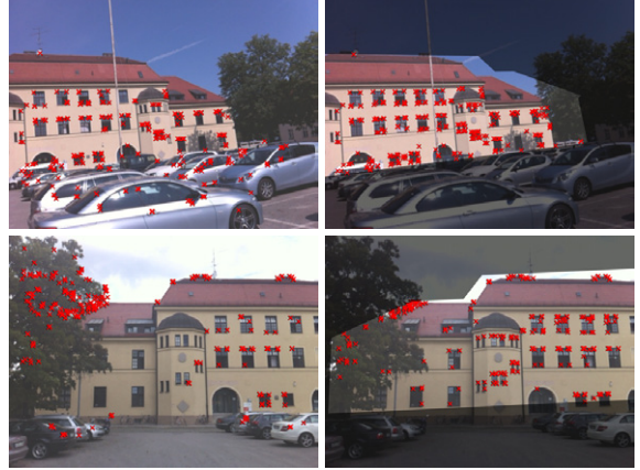
Figure 2: Comparison of regular feature detection on the entire image (left) and the proposed environment model-guided approach (right).
